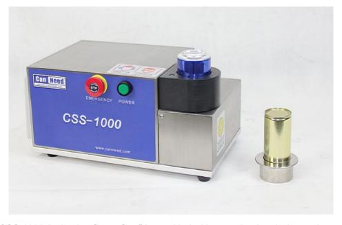
"CanNeed -CSS-1000 Anti-noise Seam Saw" is provided with an anti-noise design and a special guide for 2-and 3-piece cans with 65mm dia, such as beer cans and 209 cans. The cutting process is so precise, quick, safe and convenient to ensure precise cutting effects without distorting the cans. The seam image on Canneed series Seam Sight TM automatic seam measuring systems gets thereby every clear and improves measurement speed and reliability.
